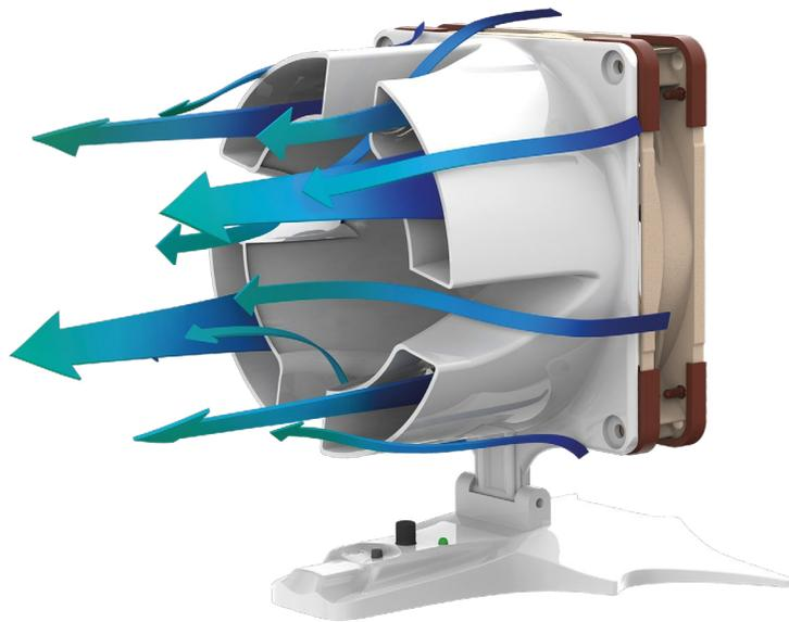
In accord with the principle of conservation of energy, air pressure must decrease as air velocity increases (Bernoulli's principle). This reduction in pressure that occurs when a fluid flows through a constriction, the so-called Venturi effect, creates a suction force at the outlet, which draws in additional air from the sides and through the cuts of the funnel, thereby enhancing the airflow volume.
